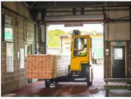
The multi-directional forklift designed for the safe, space saving and productive handling of long and bulky loads.
