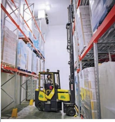
The fully enclosed, high visibility cab keeps drivers warm, reducing the time needed for breaks and increasing productivity. To improve driver visibility while performing truck to rack operations, heated cab windows eliminate the build-up of condensation when driving between different temperatures.
