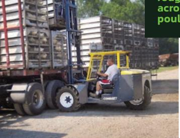
Ultra-smooth controls permit quieter, more refined handling for optimal livestock welfare. For the driver, an offset driving position affords excellent visibility while a deep suspension seat and fully enclosed cab options provide all-day comfort in any weather.
