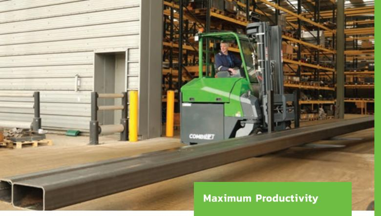
Its low profile and compact design enable the COMBi-CB to offload HGVs, bring goods to racking or to feed production lines and loading containers.
